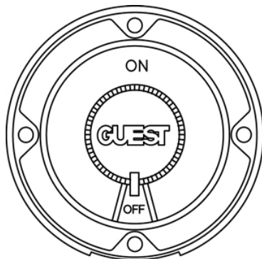
TYPICAL BATTERY SWITCH (FIG. 28.1)
